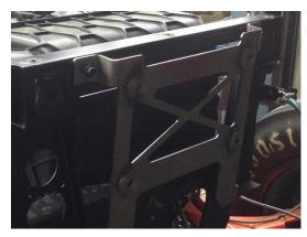
muffler and muffler bracket, you may need to loosen the head pipe bolts and swing it in the desired direction. Be sure to re-tighten the head pipe bolts before mounting the muffler\*\*\*
